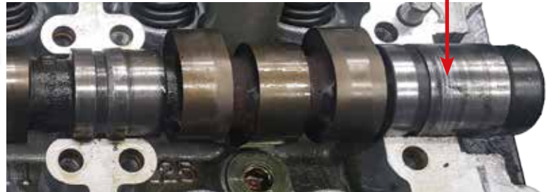
The bearing surface of the camshaft has been damaged from lack of lubrication on start-up.
