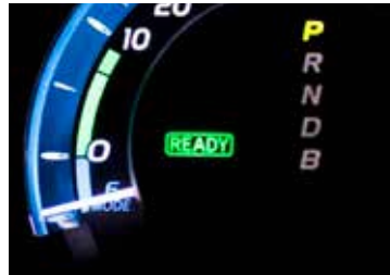
This is the 40 series "READY" light, it indicates that the vehicle is powered up and ready to drive.
