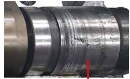
The bearing surface of the camshaft has been damaged from lack of lubrication on start-up.
